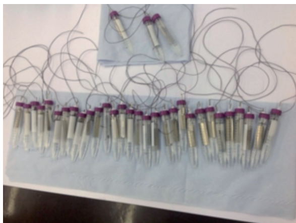
Fig. 3. Titanium plate inserted centrifuge tubes filled with water.
